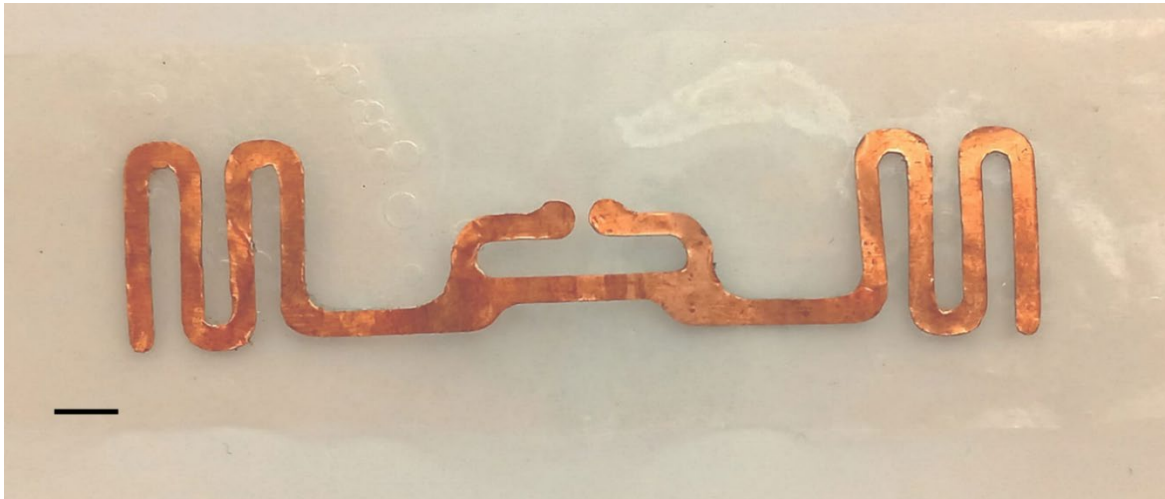
Figure 3.12. Optical image of an UHF copper antenna on chitosan substrate. The scalebare is 5 mm
