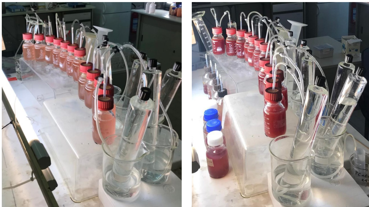
Figure 22, Bottle configuration at the beginning (left) and end (right) of phase 2
