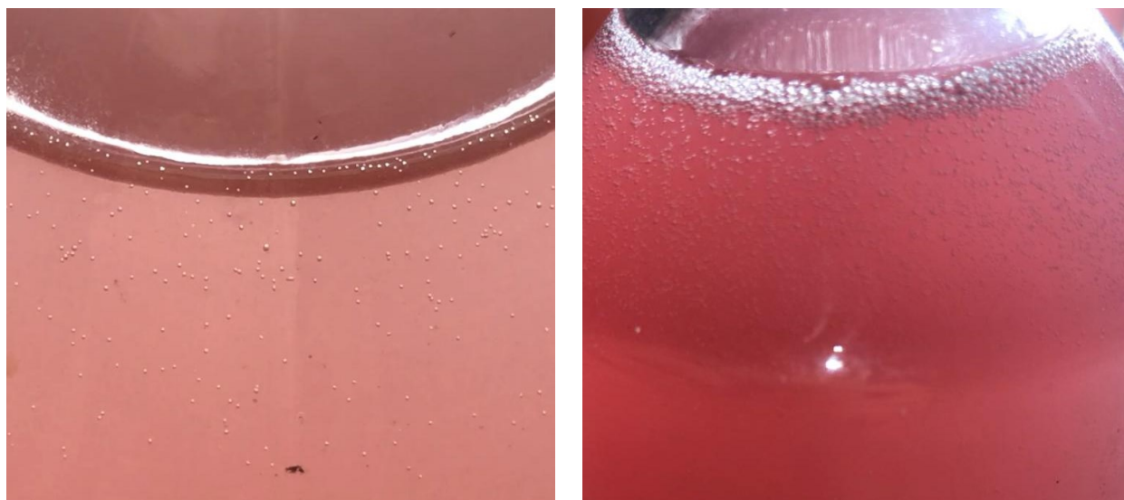
Figure 21, Detail of hydrogen bubbles formation in the test bottles during phase 1
