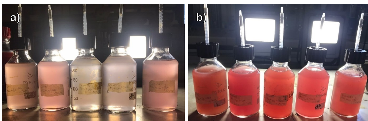
Figure 18, Rps. palustris strains growing on RPN medium a) immediately after inoculation and b) before transferring the strains onto RPP. In each picture, from left to right: Rps. palustris 42OL, not used in this experiment; Rps. palustris CGA009; Rps. palustris CGA4001; Rps. palustris CGA4013; and Rps. palustris CGA4017.
