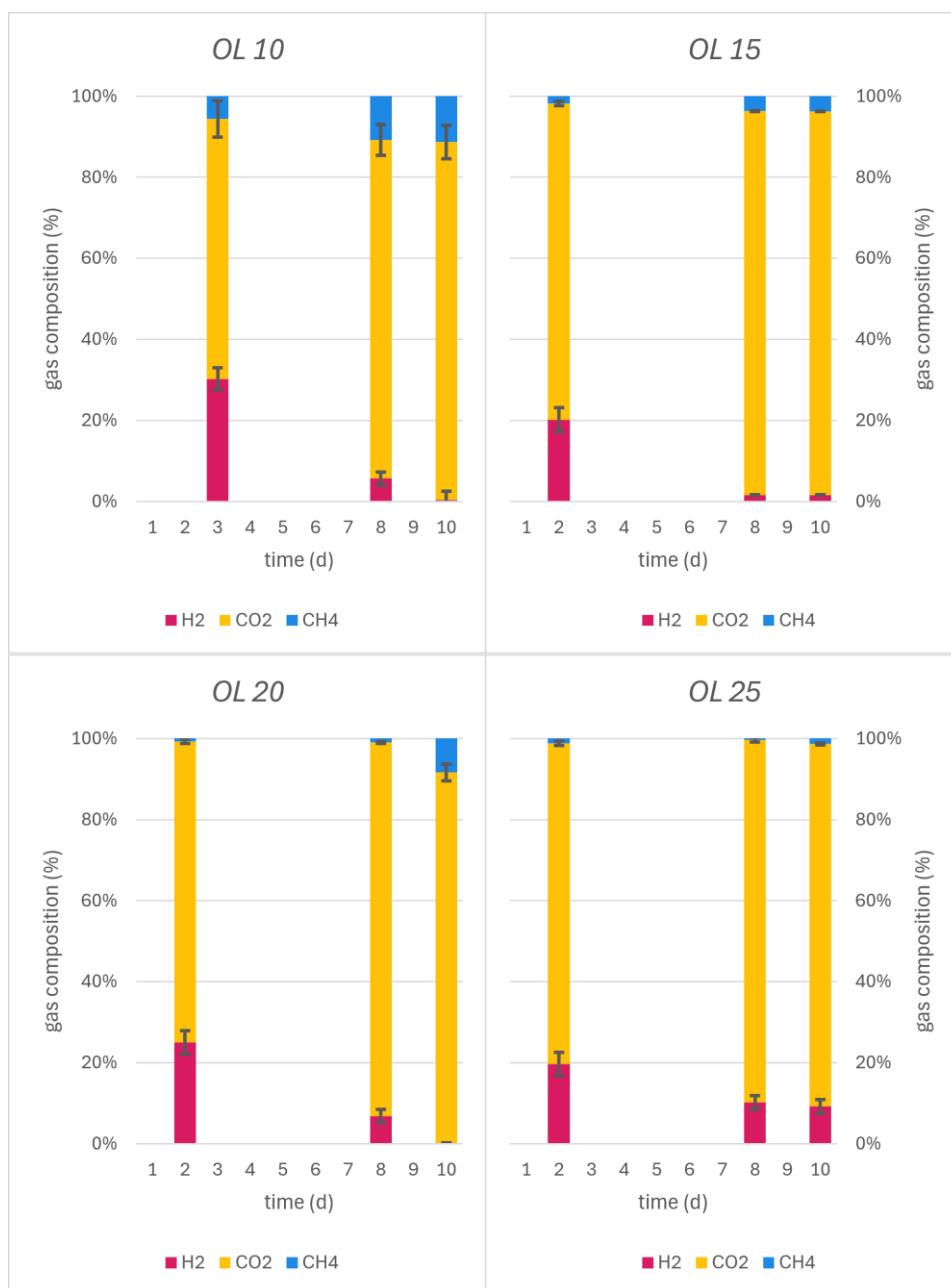
Figure 27, Composition of the produced biogas during Test 1
