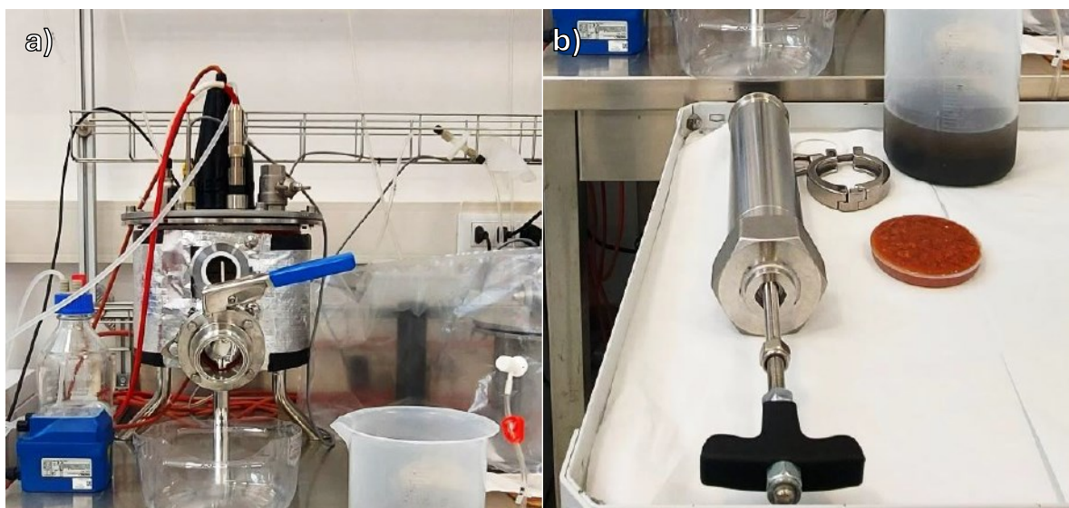
Figure 9, Modified vessel employed in Test 3. a) detail of the charge/discharge valve; b) syringe used for effluent removal and substrate addition
