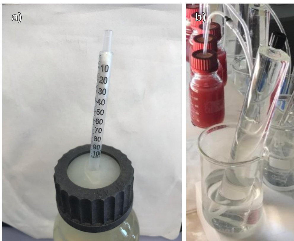
Figure 19, a) detail of the cap to allow culture sampling and gas outflow; b) gas-trap for volumetric hydrogen quantification, with detail of the one-way valve installed in between the bottles and the gas-trap during phase 2
