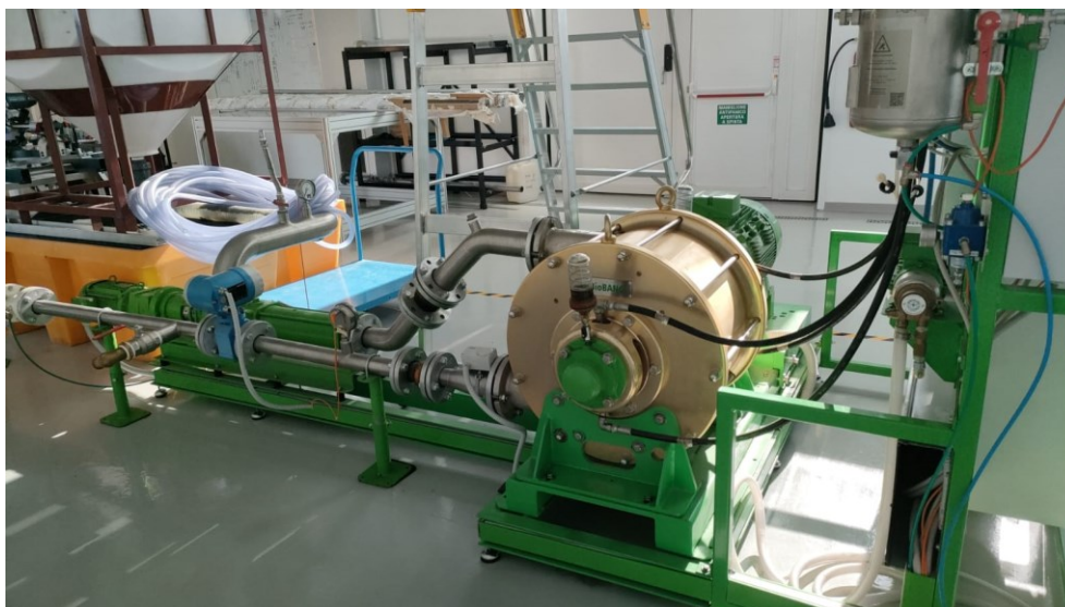
Figure 8, Hydrodynamic cavicator employed for the HC pretreatment
