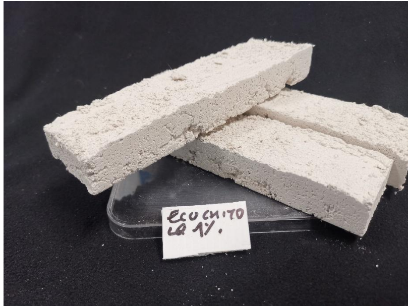
Figure 56 Close up of sample E_CL1, it is noticeable the presence of voids in the sample matrix
