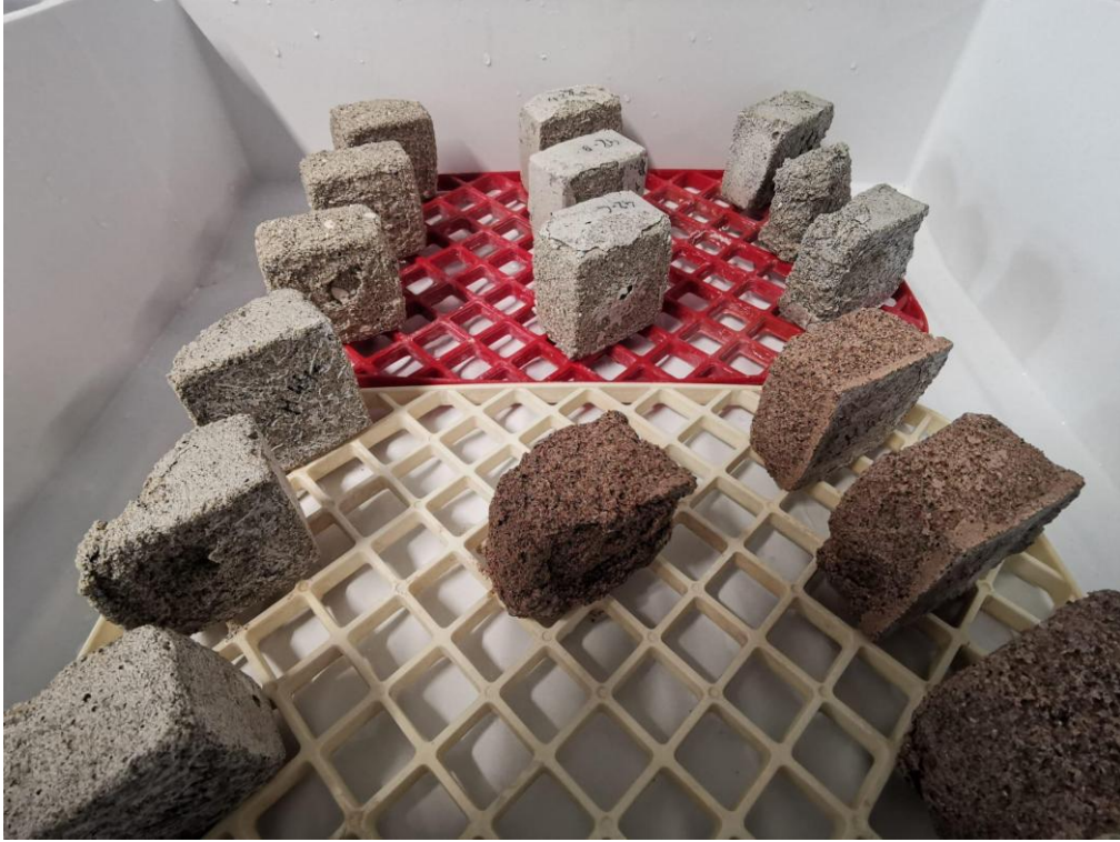
Figure 7 Mock-ups undergoing freeze/thaw cycles
