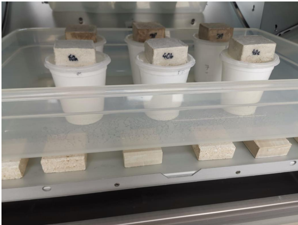
Figure 6 Mock-ups inside the climate chamber for ensuring the controlled environment
