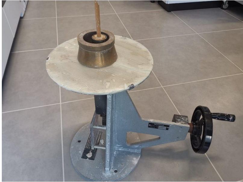
Figure 4 Shock table used for the test
