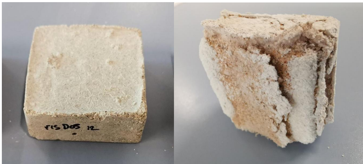
Figure 51 Samples LSC_D05 before and after salt cycles.
