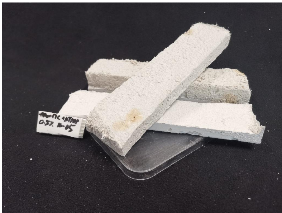
Figure 59 Sample of RMC_D05 with detachment between parts of MC and Rinzafo
