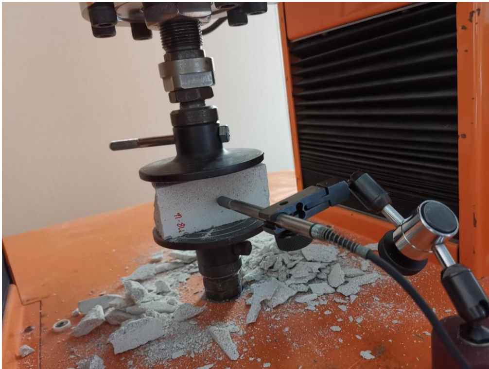
Figure 9 Mock-up undergoing compressive strength resistance evaluation with additional (side) probe for monitoring its integrity
