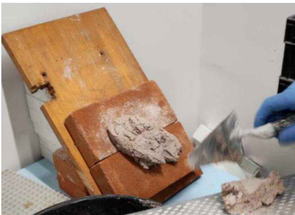
Figure 60 Evaluation of fresh mortar workability on tilted surface
