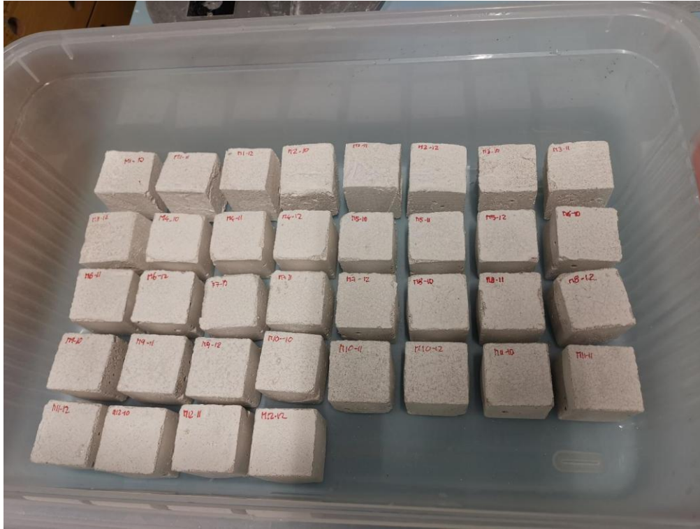
Figure 8 Cured cubic mock-ups used for the resistance to soluble salts test
