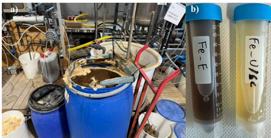
Figure 6.9: Fenton process dosage (a), influent, and clarified effluent of the Fenton process (b).
