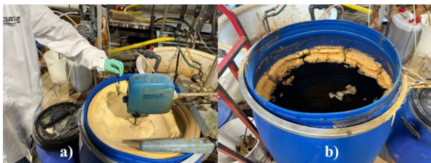
Figure 6.6: Fenton process agitation phase (a) and precipitation phase (b)
