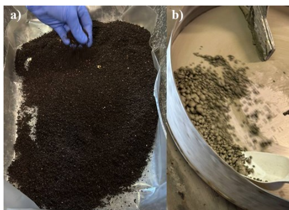
Figure 6.10: Sludge resulting from the Fenton process after dehydration (a) and granulation (b).
