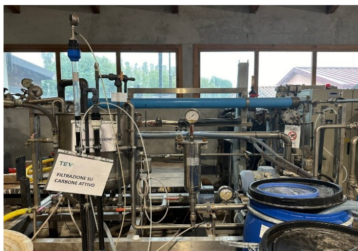
Figure 6.3: Nanofiltration using the membrane NF270
