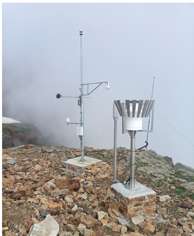
Figure 8 - The Passo dei Salati Station. The two rain gauges are visible in the foreground (weighing and, behind it, the tipping bucket); in the background is visible the pole with the anemometer (top of the pole), the snow meter (right branch), the RoX (upper left branch), and the thermo-hygrometer (lower left branch).
