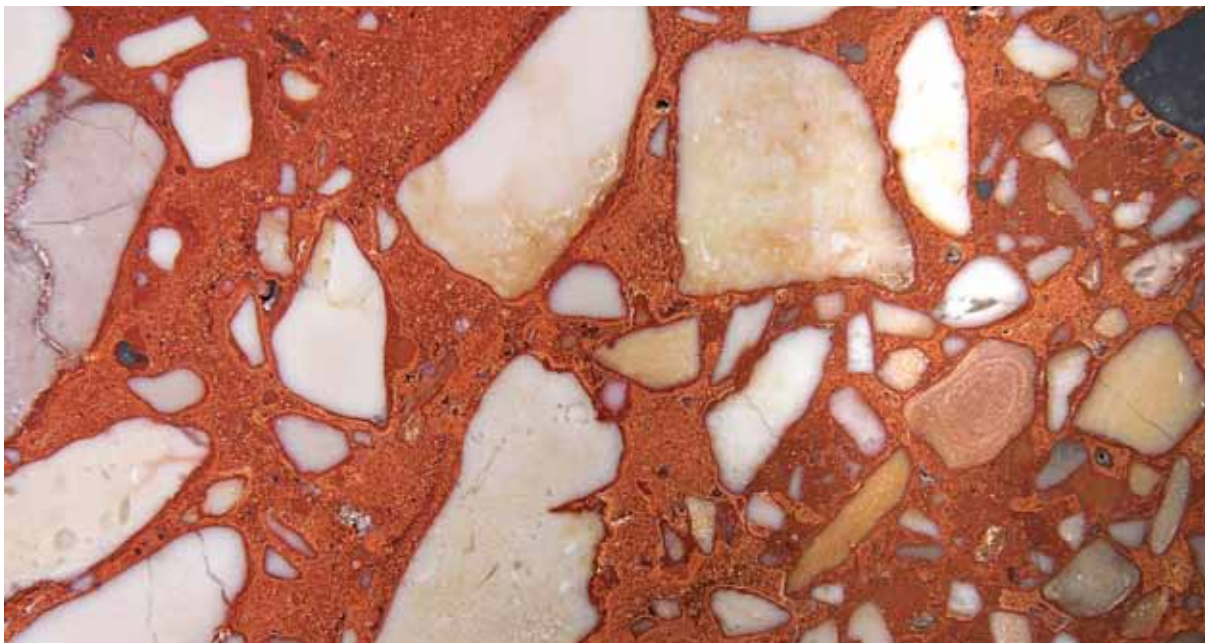
Fig. 3 - The typical macroscopic aspects of the breccia rossa e gialla egiziana with abundant beige subangular clasts and a few ones of dark grey and pinkish color in a brick-red cement
