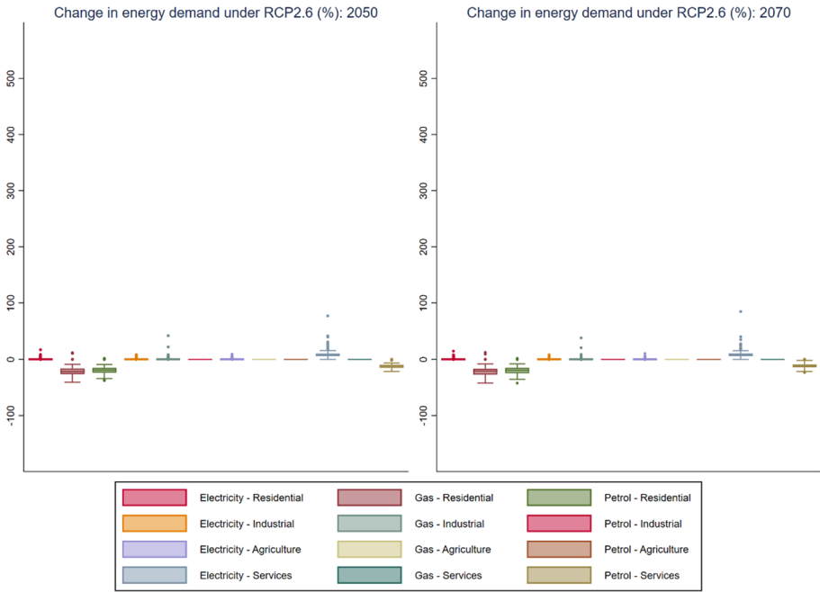
Fig. 10 Box-plot of climate-induced energy demand trends in EU regions and RCP2.6 (2015–2050% changes left, 2015–2070% changes right)
