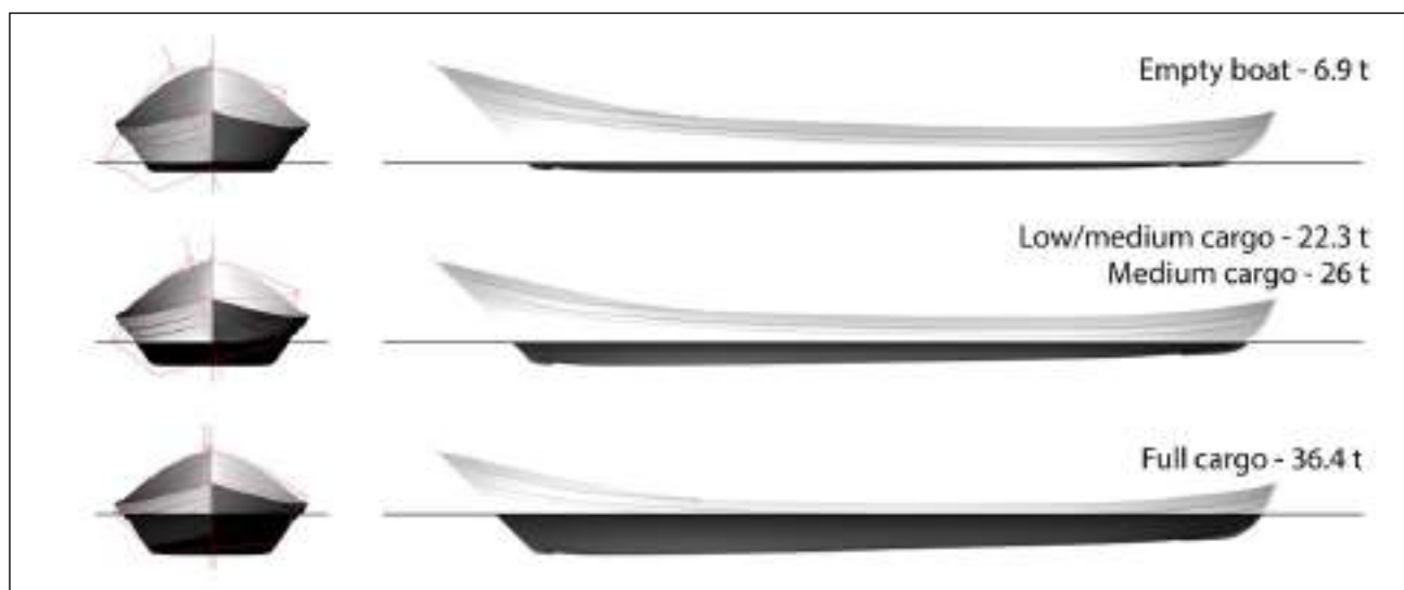
Fig. 13.3. Comparison of water level and stability with three different cargo conditions. a. Empty boat. b. Low/medium and medium cargo. c. Full cargo (elaboration: E. Costa).
