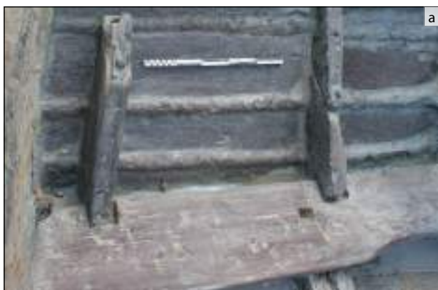
Fig. 9.22a-b. The L-shape recess with two holes near the stern (photo: E. Costa).
