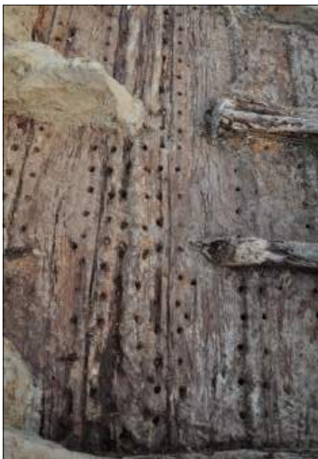
Fig. 9.3. Longitudinal fracture on plank P3 repaired with the sewing technique (photo: E. Costa).
