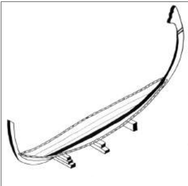
Fig. 14.1. First phase of the 'shell-first' method.
