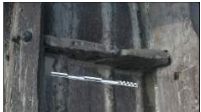
Fig. 9.19. One of the futtocks connected to the frame with iron nails (photo: E. Costa).
