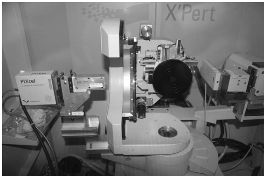
Fig. 3 The diffractometer-token used at the IJL
