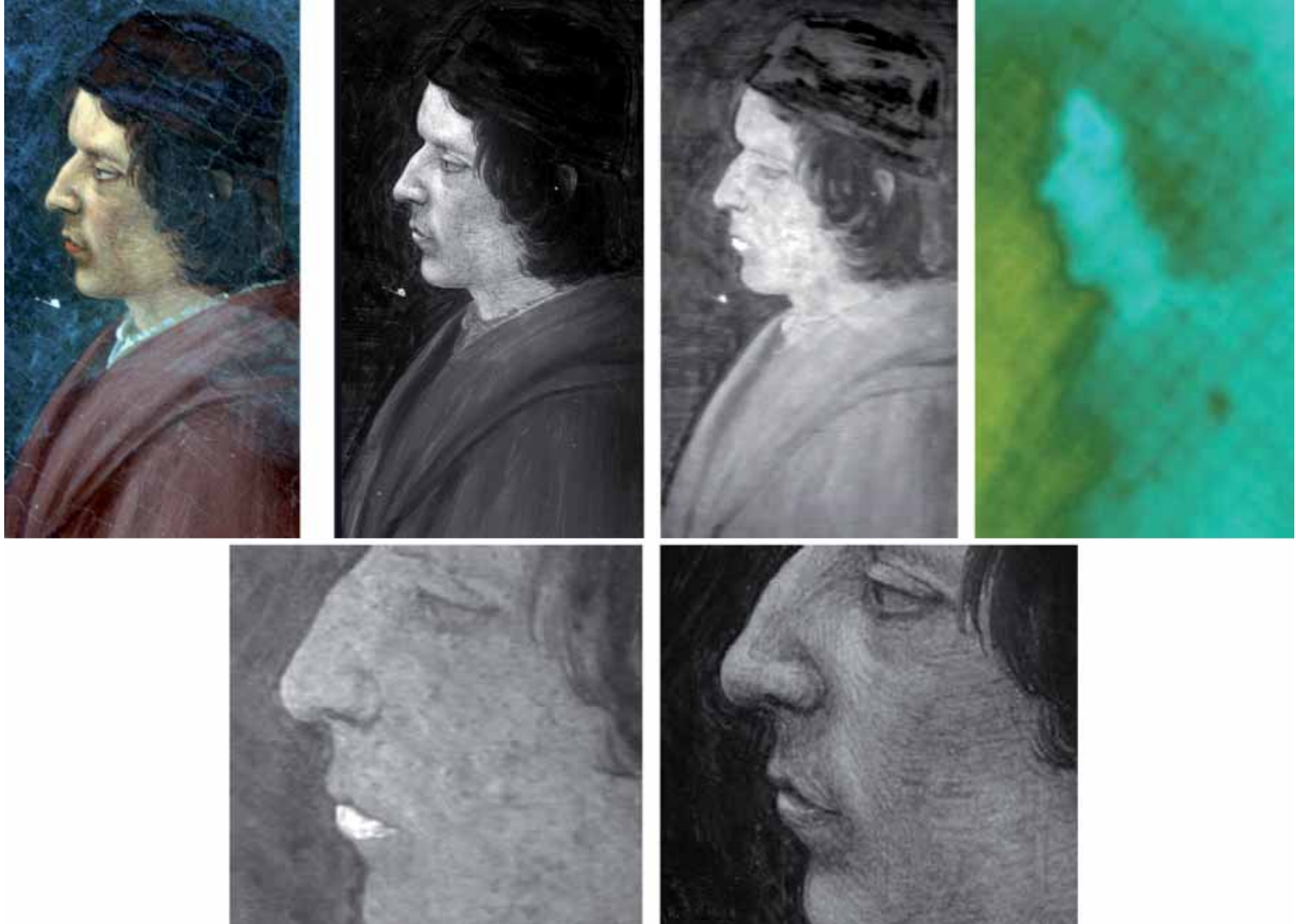
Figure 3. Analysis of a fresco model (OPD laboratories). From the left: VIS image, near-infrared reflectography (1 \mu m Si CCD), TQR image (3-5 \mu m), far-infrared thermography (thermogram after heating pulse). The detail: mid-infrared TQR (left), near-infrared scanner reflectography (2.2 \mu m)
