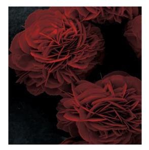
**Fig. 7.** False-colored scanning electron microscopy image of hybrid protein-inorganic nanoflowers.
