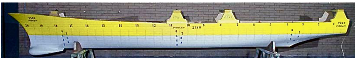
Fig. 7. A 5.720 m length model of the DTMB 5415 (CNR-INM model 2340).
