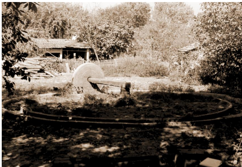
Figure 6. Hard fruits were smashed with special machinery similar to a mill wheel (Hungary), called as “almatörő járgány” (apple-cracker capstan). (Picture is from the archive photo gallery of Janus Pannonius Museum, Pécs, Hungary).
